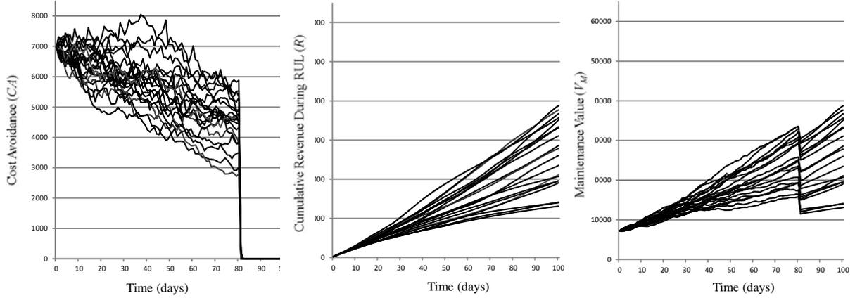
**Figure 2. Propagation of the properties in Figure 1 in time with uncertainties. In this example, the RUL is 100 days and 20 paths are shown. Note, the properties also include a jump to zero in the cost avoidance at 80% of the RUL.**
