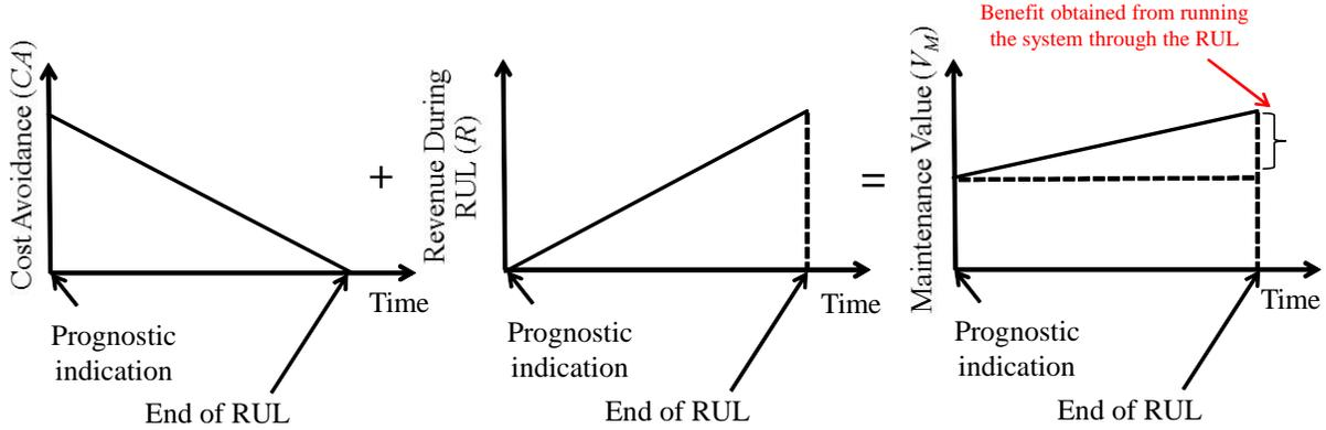
**Figure 1. Value of waiting to maintain. This simple representation assumes that the severity of the failure is constant but the probability of failure increases as the RUL is used up. This figure does not address uncertainties in the RUL.**
