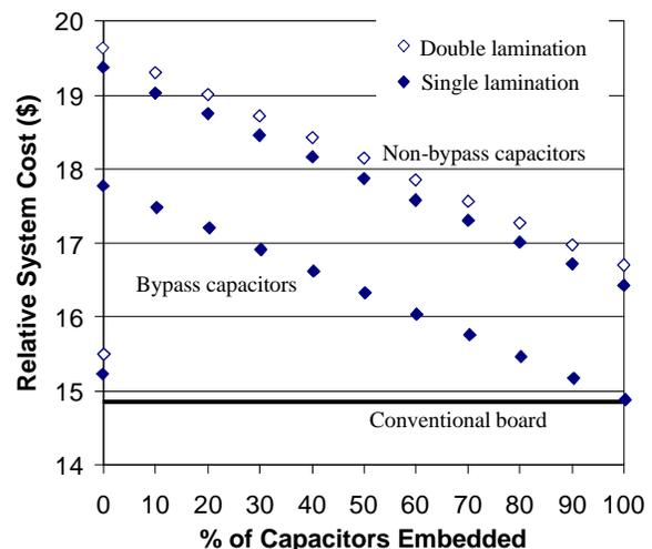
Figure 5. Capacitor embedding for the picocell board application.
