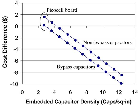
Figure 6. The impact of embeddable capacitor density on system cost for the picocell board application.
