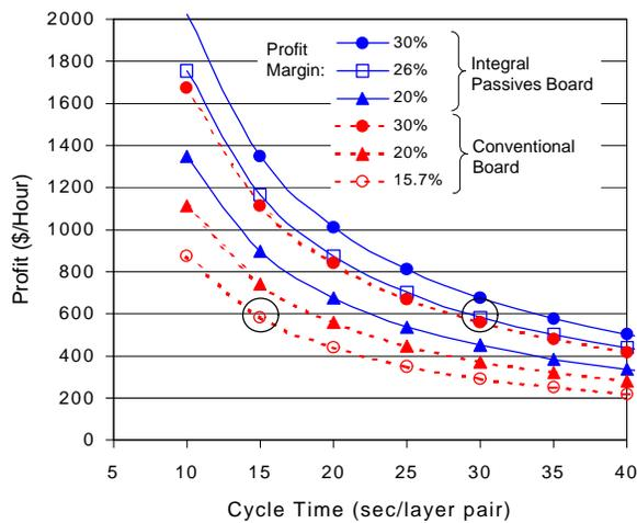
Figure 2 - The relationship between profit margin and production cycle time for conventional and integral passive board fabrication.
