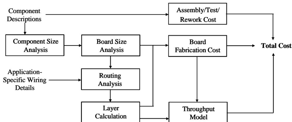
Figure 1 – Summary of cost model developed for the analysis of integral passive cost impacts on electronic systems, [10].
