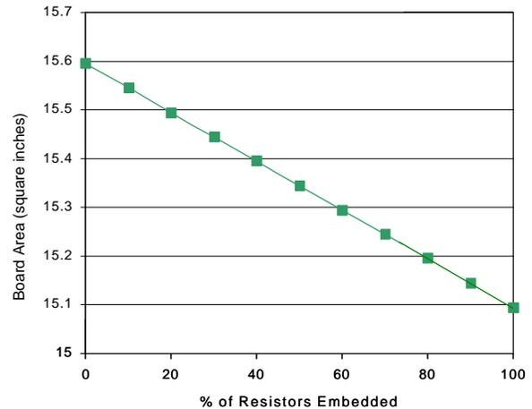
Figure 4. Board size decrease with resistor embedding for picocell board application.
