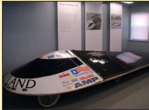
Left: The award winning solar-powered car 'Pride of Maryland', which blends bicycle and airplane technologies to create a lightweight, aerodynamic, non-polluting vehicle.
