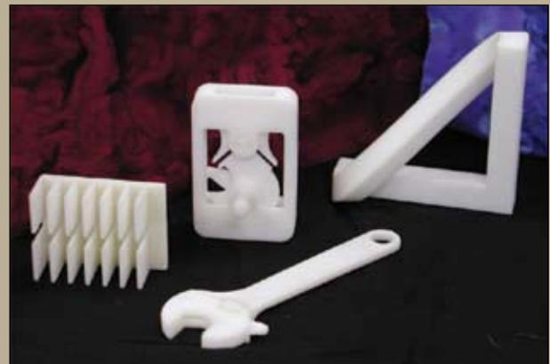
Above: Plastic objects created by the rapid prototype machine, initially created with a computer-aided design (CAD) program. The machine can create single parts or whole, functional devices for product realization.
