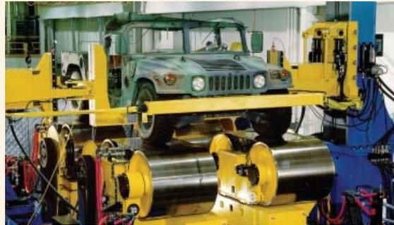
Vehicles tested on the Roadway Simulator ride on treadmill-like actuators that measure vertical, cornering and traction capabilities
