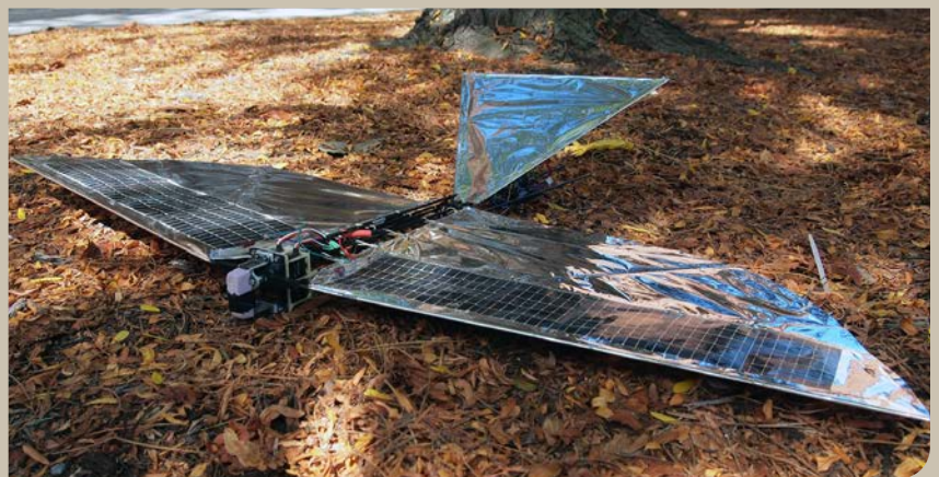
ROBO RAVEN III IS THE FIRST FLAPPING WING MAV IN THE WORLD THAT FLIES ON BATTERIES CHARGED BY ONBOARD SOLAR CELLS.
