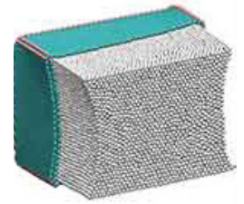
HYDROGEN (WHITE) IS PACKED INTO A TINY BOX MADE OF GRAPHENE, WHICH RESEARCHERS AT THE UNIVERSITY OF MARYLAND CAN OPEN AND CLOSE USING ELECTRICITY. CREDIT: MARYLAND NANOCENTER
