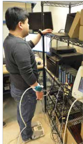
The weighing scale-like system can calculate pulse transit time.
