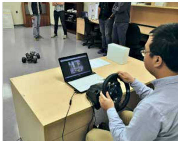
Using a steering wheel and foot pedals, this driver operates a scaled-down vehicle remotely.
